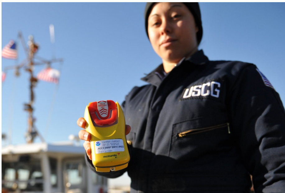
Seaman Asleigh Wilson, a boatcrew member at Aids to Navigation Team Baltimore, holds a personal emergency position indicating radio beacon on a pier located in Curtis Bay, Md., Dec. 9, 2010. Crewmembers at ANT Baltimore carry PEPIRBs while servicing aids throughout the upper Chesapeake Bay. U.S. Coast Guard photo by Petty Officer 3rd Class Robert Brazzell.
