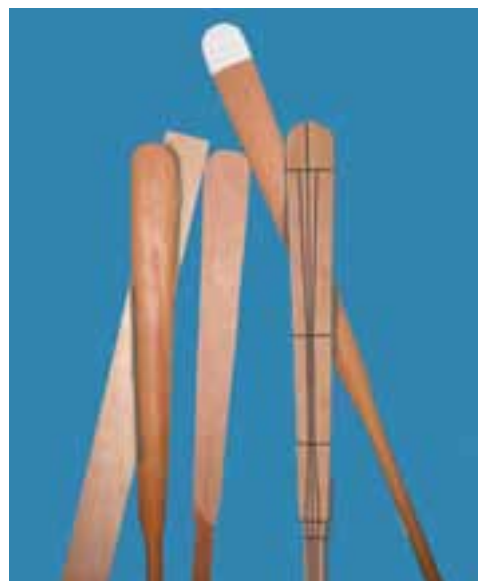
Front row L-R: Finished storm paddle, paddle blank, blank with marks for planing. Back L-R: fir 2X4, finished paddle.
