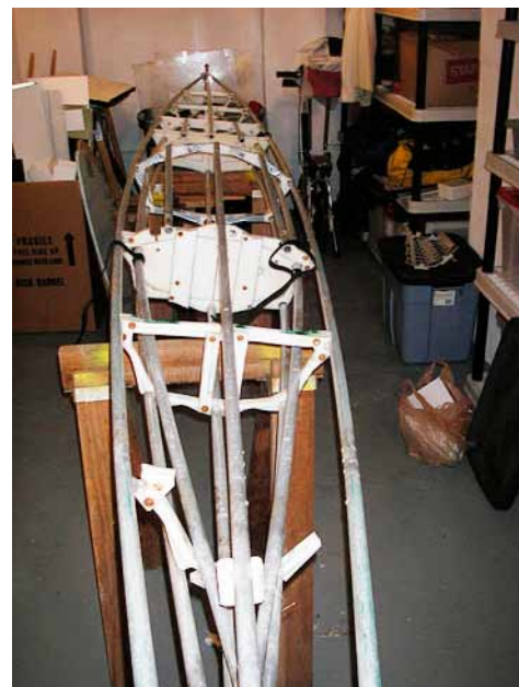
Looking aft along the deck ridge. Note broken frames.
