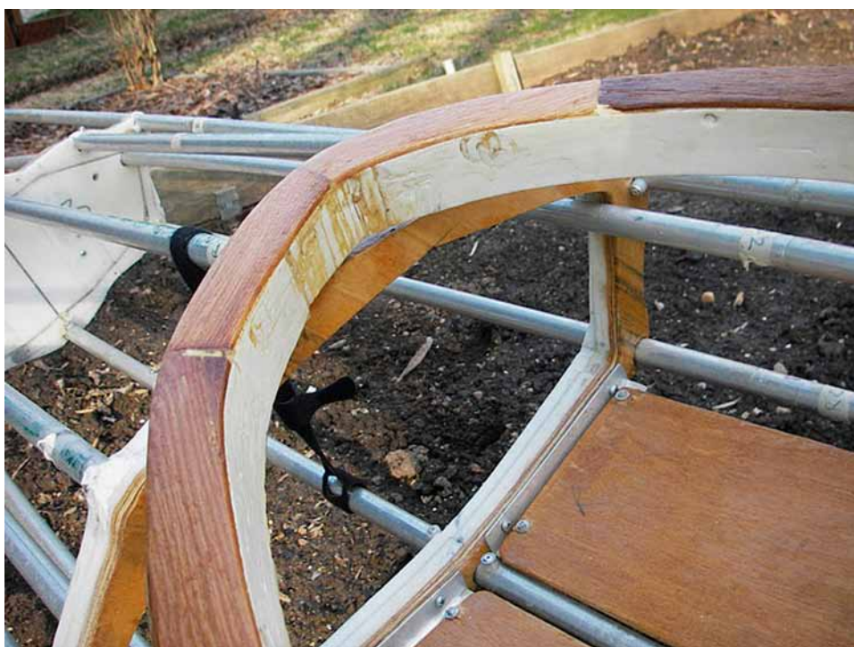
Floor board and rim detail, Note riveted aluminum angle irons to support the boards.
