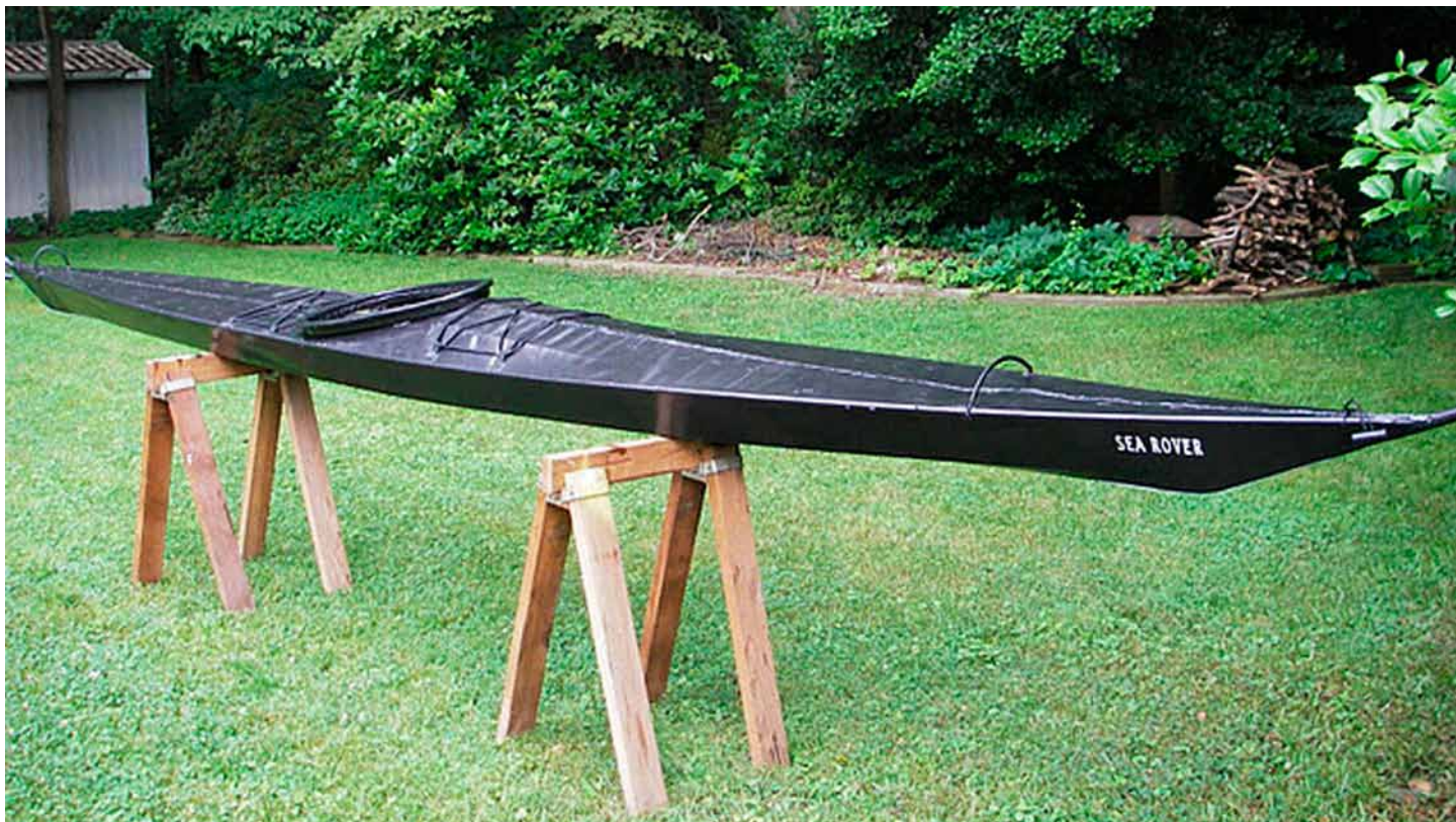
The finished Yost Sea Rover Greenland skin-on-frame kayak.
