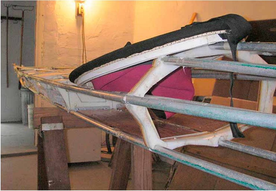
Though out of sequence, this image shows the steep angle of the cockpit rim.
