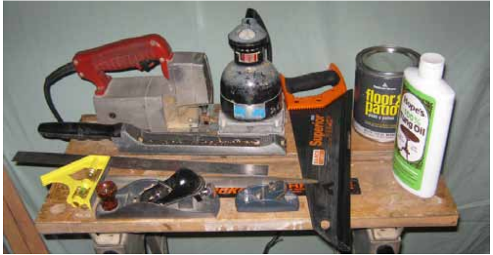
The tools. Left to right, back to front: saber saw, orbital sander, hand saw, epoxy-fortified paint, tung oil, combination square, medium rasp, block plane, mini plane.
