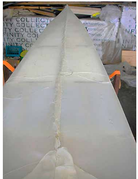
The finished bow seam. I sewed the seam using a curved upholstery needle.
