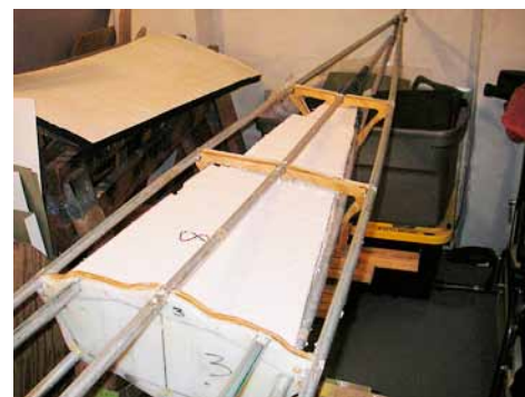
The foam blocks installed in the bow.
