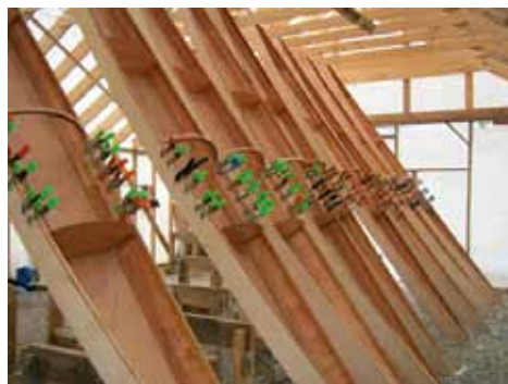
The cockpit reinforcements are clamped up and drying.
