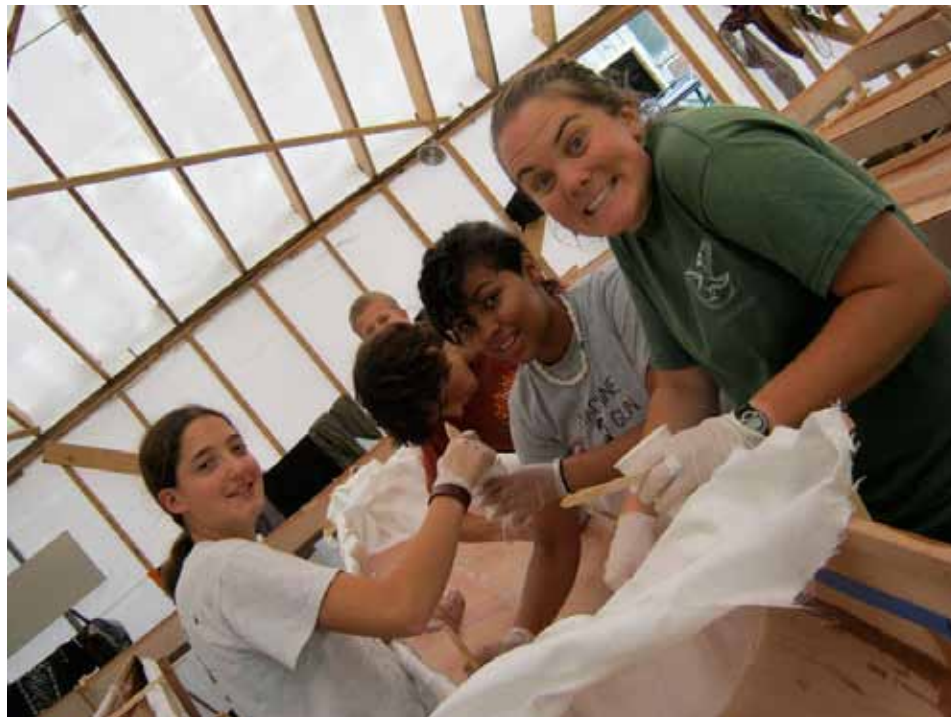
Emma helps Nadine, Antoine, and Chevella to line a hull with fiberglass.
